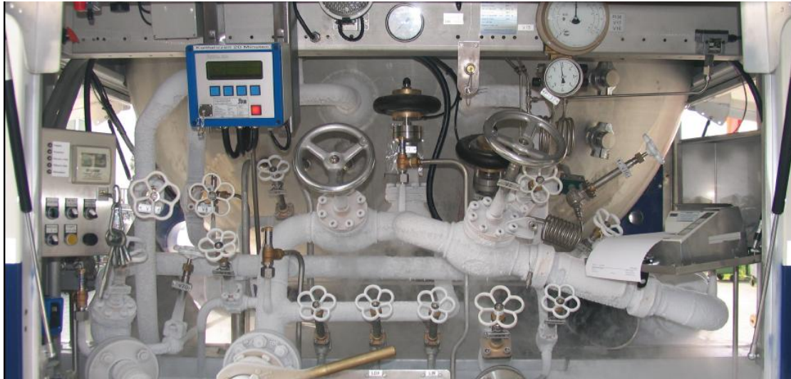
Caption: The Flowcom 2000™ Cryogenic metering system being supplied by Cryoshield.
