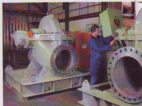
Split-case pump typically used in mine-processing applications
