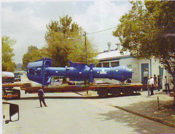
1600mm APE vertical turbine pump
